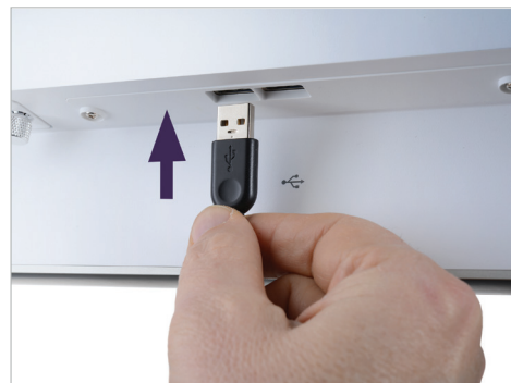
12. Plug in the webcam to the USB port at the bottom of the HD screen
