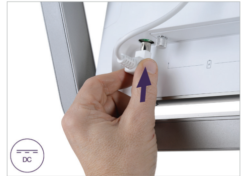
14. Attach the power cable to the port labeled DC
