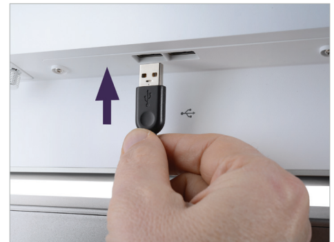
23. Plug in the webcam to the USB port at the bottom of the HD screen
