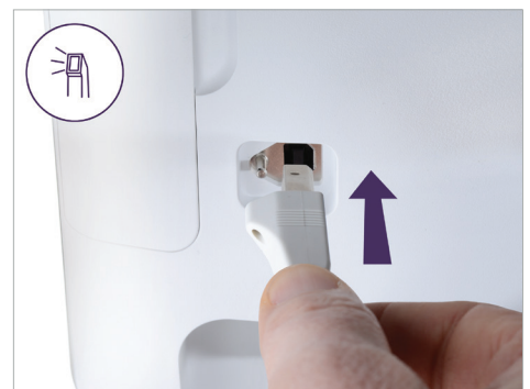
9. Attach the wand cable on the back of the HD screen
