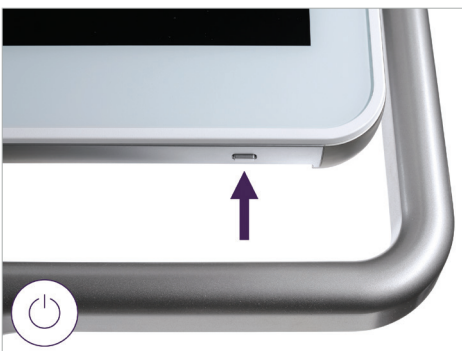
24. Press button to switch on the scanner
