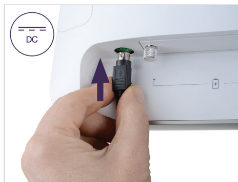
8. Attach the power cable to the port labelled DC
