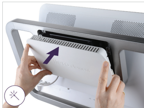
16. Attach the magnetic back cover
