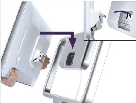
12. Lift the HD screen to mount it
