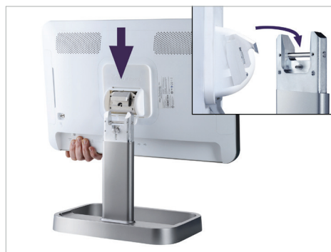
5. Lift the HD screen to mount it.
