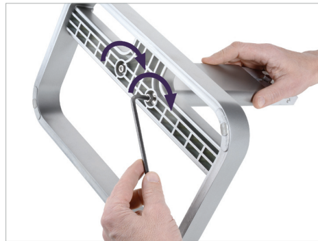
2. Tighten the post using the allen wrench
