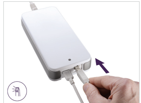
5. Connect wand cable to the hub
