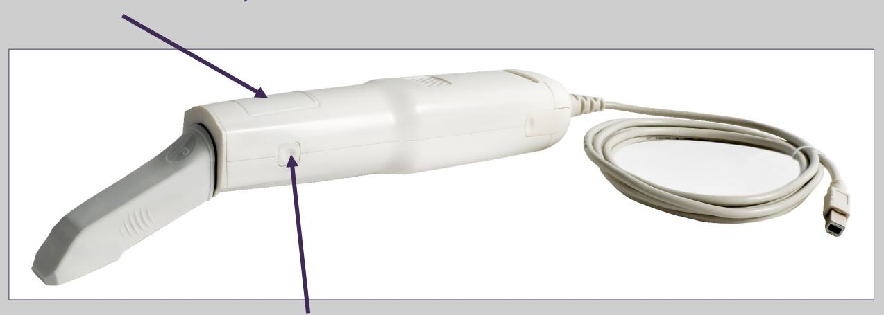
To start and stop scanning, press and release either of the side buttons.
